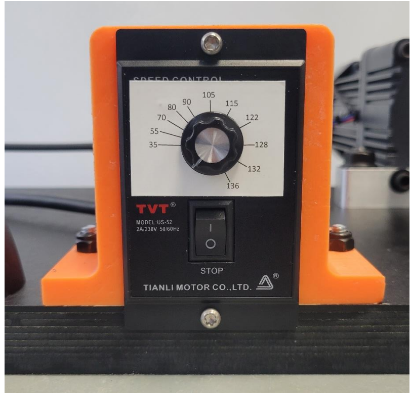
Motor speed control with calibrated bpm increments.
