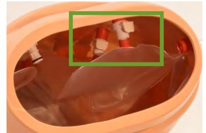
9. Remove the reservoir by pressing the push connectors
