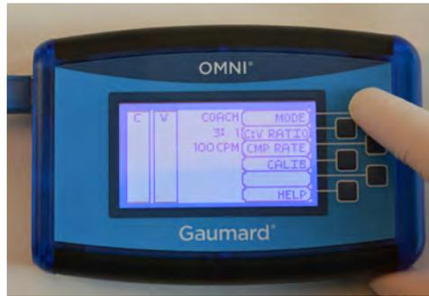
**WARNING: Do not connect the Blood Pressure Arm or Omni to a computer, LAN network or unauthorized diagnostic equipment using the communication cable (Ethernet cable). Doing so will cause serious damage to the equipment.**
