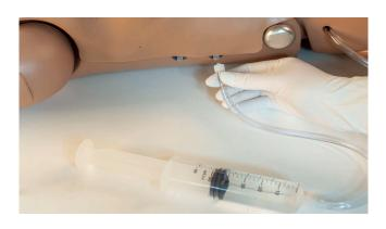
4. Connect the drain hose to the other port and place the end of the hose into a receptacle.
