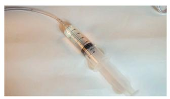
3. Connect the fill syringe to one of the ports on the right side of the simulator.
