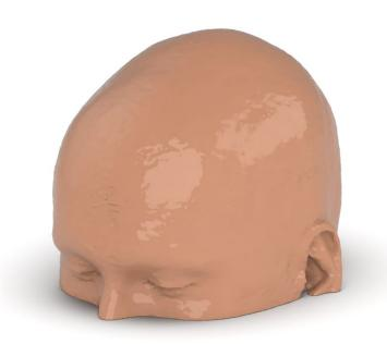
This phantom simulates a contrast medium enhanced head in arterial phase (CT angiography). It covers the vertex to the foramen magnum.
