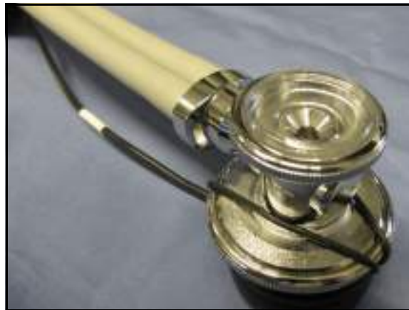
StethoSym Speaker Module Connected to Diaphragm
