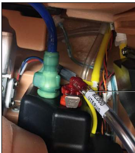
The Lower Baffle Ports
