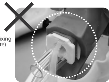
Example of inappropriate installation of tongue component
