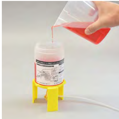
2) Pour in over 600ml of liquid into the container. Put the lid back on to prevent spilling.
