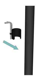
14 | Just so that we know where they are for later, identify the two Allen keys along with the push fit clamp provided. Snap this to the post and move to the next step.
