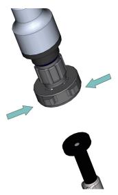
31 | Connect the camera coupler to the laparoscope by pinching the two clasps. It should lock into place firmly.
