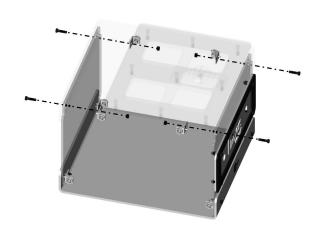
7 | As in Steps 1 and 2, secure the TPB05 sub-assembly to the upright panels using: 4 x MA01, 4 x M529 bolts and 4 x WN29 nuts.
