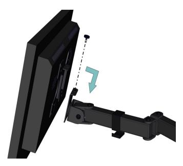
20 | Slide the monitor into position and screw the bolt into place.
