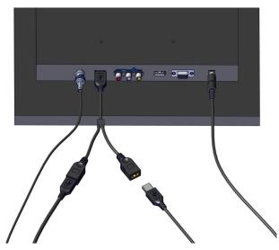
27 | Connect the USBA/B cable to the remaining USB port on the USB splitter.
