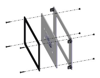
9 You may now start the side panel sub-assemblies. Taking SPBL, SK07 and BKT06, secure as shown using 4 x M529 bolts and 4 x WN29 nuts.
