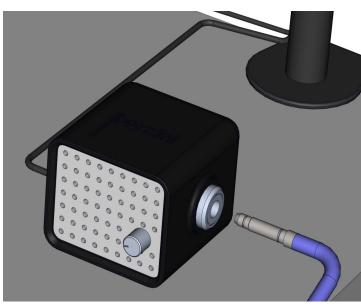
29 | Plug in the male end of the fibreoptic cable into the light source.
