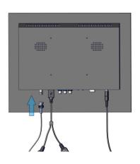
22 | Plug the socket into the wall and then Connect the IEC cable to the power adapter. When switched on, a green light may be shown.
