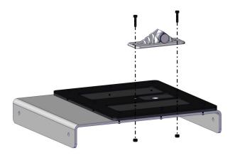
6 Isolate the scope bracket (INO-BLBKT). Using 2 x M529 bolts and 2 x WN29 nuts, secure the bracket as shown in the image.
