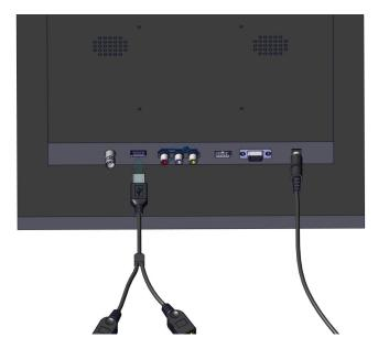
23 | Connect the USB splitter to the rear of the monitor as shown.
