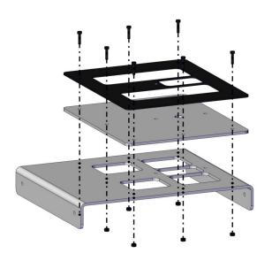
5 You may now start the TPB05 sub-assembly. Taking TPB05, SK08 and BKT07, secure as shown using 7 x M5B29 bolts and 7 x WN29 nuts.
