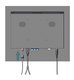
25 | Connect the female end of the BNC extender to the screen.
