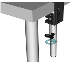
18 | With the bracket fully assembled, anchor it to your chosen work surface by turning the handle until it is tight.
