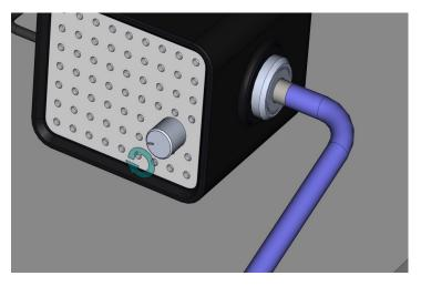
30 | When the screen is powered on, you should be able to turn the knob on the front of the light source to activate the light. Test the light at this stage and switch off.
