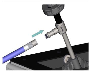
33 | Attach the other end of the fibreoptic cable to the connector on the scope by screwing it into place. At this stage, you are ready to turn the light source on.
