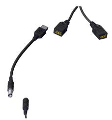
24 | Connect the USB to 5V adapter to one of the USB ports. Connect the female end of the BNC cable to the male end of the 5V adapter.
