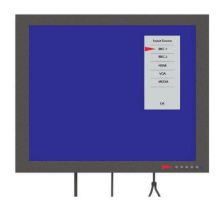
35 | In most cases, your monitor will have been pre-programmed to display the image. In the event that you do not have an image on screen, push the left most button on the screen and select BNC1. Once the image appears you are now ready to operate.
