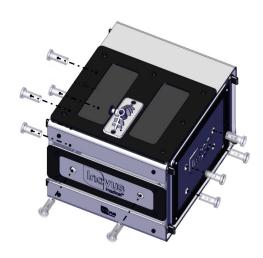
11 | Insert the 10 dummy trocars as directed in the image.
