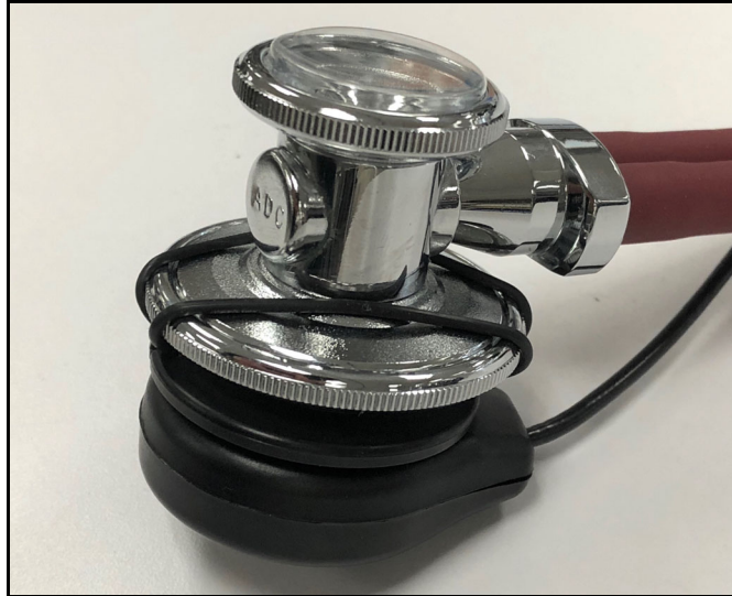
StethoSym Speaker Module Connected to Diaphragm
