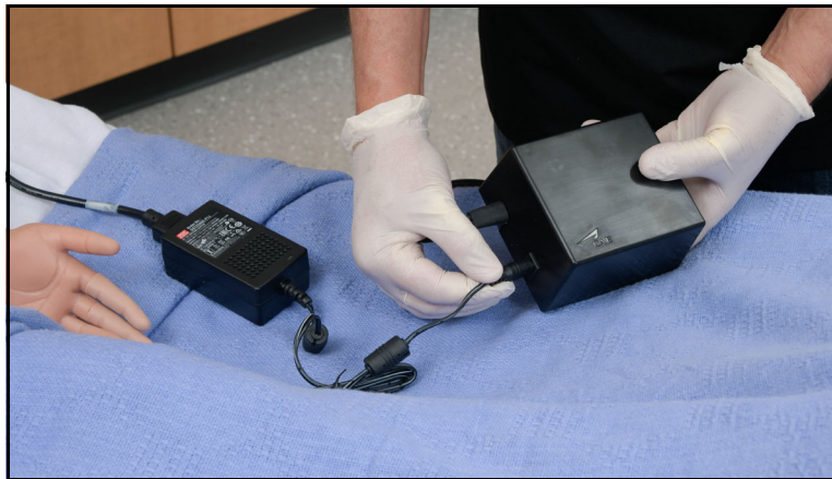
Charging the SymDefib
