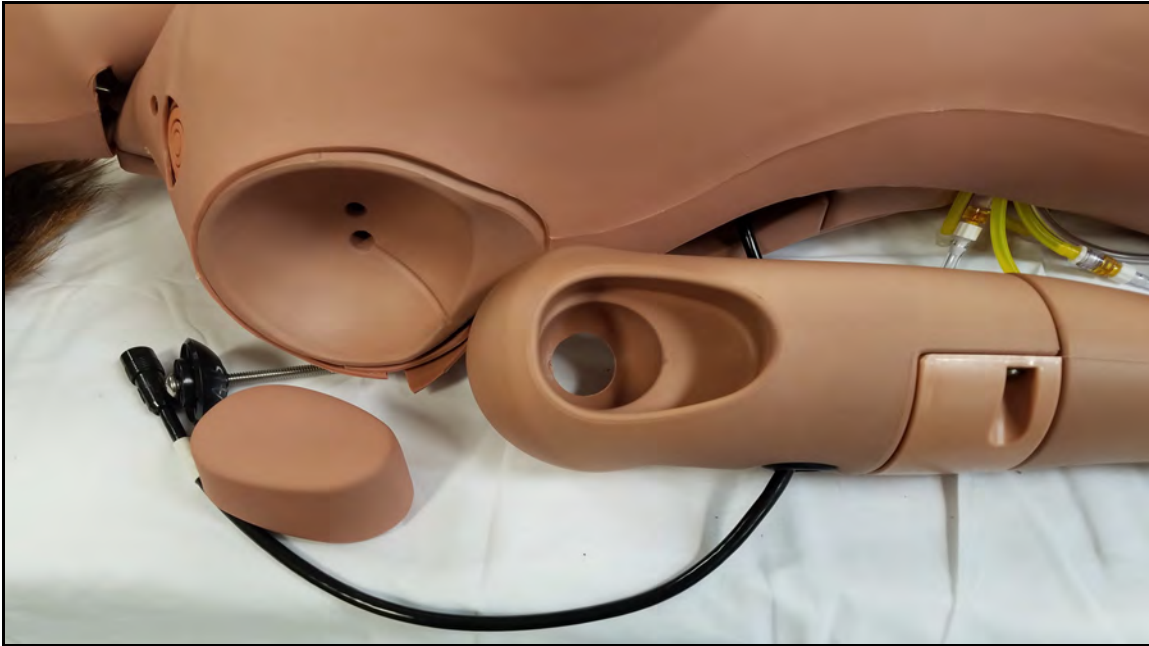
The NIBP Arm IM Pad Removed and NIBP Arm Ready for Installation
