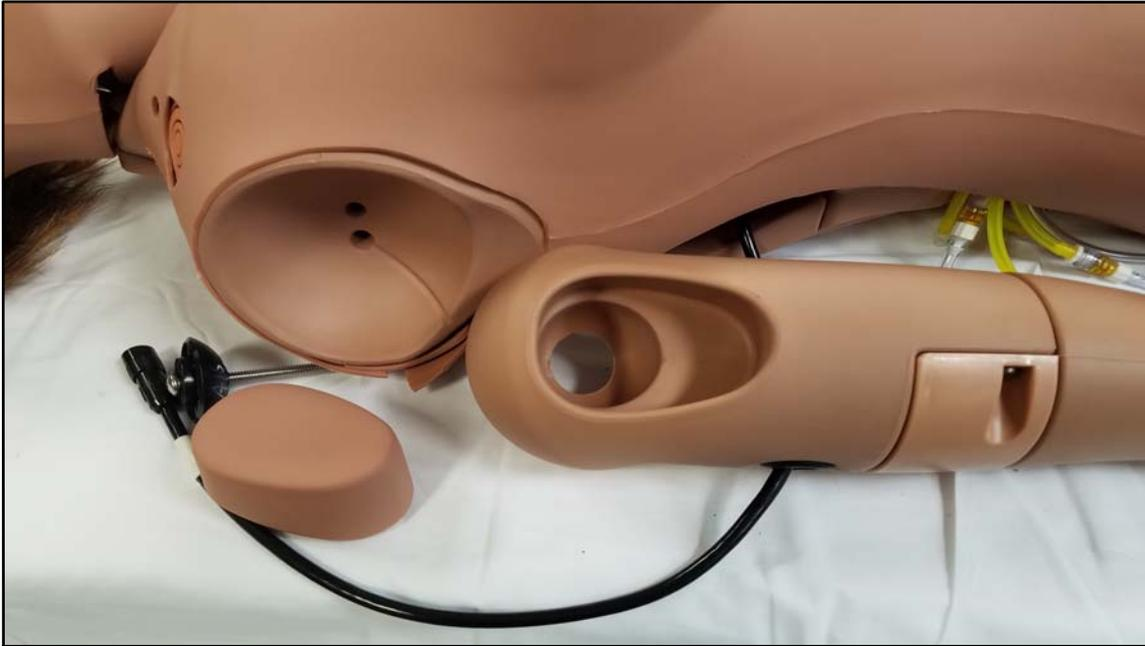
***The NIBP Arm IM Pad Removed and NIBP Arm Ready for Installation***
