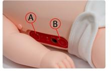
A: + and – allows ventilation feedback to be audio and/or lights. B: Scenario button switches on brachial pulse.
