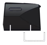
2 With the acrylic plate positioned half way into the drip tray, place the U-shaped bracket onto the plate and align the two circular bolt holes on the bracket with those on the plate.
