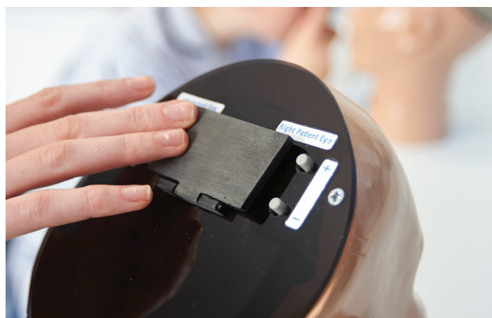
Cover to hide condition LED indicators under examination conditions
