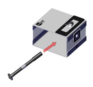
11 | You may now position the scope to begin training. The scope must be placed backwards through the ports, as illustrated. Positioning the scope in this way reduces the risk of skin tearing.
