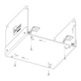
6 | Using 4x M5B24 screw each AR20\_M-BKT into position on the base. These parts are threaded for ease of assembly.
