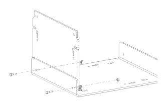
3 | Screw into place 2x MA01 using 2x M5B24 and 2x WN14
