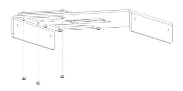
9 Now attach 3x WN14 to the bolts coming through the bottom surface. Repeat this process on the opposite side to complete the assembly.
