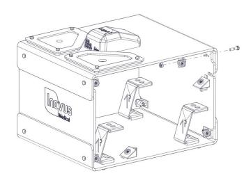
13 Using 4x MA01, 4x WN14 & 4x M5B24, repeat the process from steps 2,3 & 4. Do this on each corner so that a magnet is in place for the side panels to connect into.
