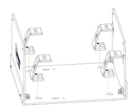
5 | Take 4x AR20\_M-BKT, position them in the keys provided. In a practical sense this will need to be done one at a time with the simulator positioned on its side.
