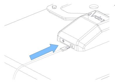
17 | Connect the USB micro into the back of the camera.
