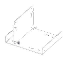
2 | Now take the following parts 2x MA01, AR20\_U02, 2x WN14 & 2x M5B24. Using the image as a guide, pay close attention to the part orientation in this step or you will have to undo work at a later stage.
