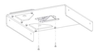
11 | Take 2x M5B24 bolts and affix the AR20\_CAM into position. DO NOT plug-in at this stage.
