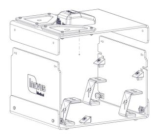
12 | Take the sub-assembly from the last four steps and place it over the upright panel of the simulator as shown.
