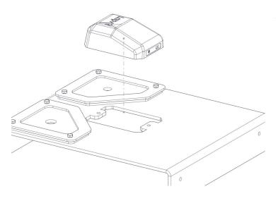
10 | Remove the AR20\_CAM from its packaging and place into positon as shown.
