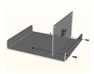
1 Begin the assembly by taking out parts UHD and BTM01. Using 2 x M5B8 bolts and 2 x WN14 nuts, screw the UHD panel into position as shown.
