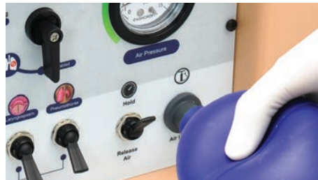
Air reservoir is charged using the supplied manual pump or a BVM
