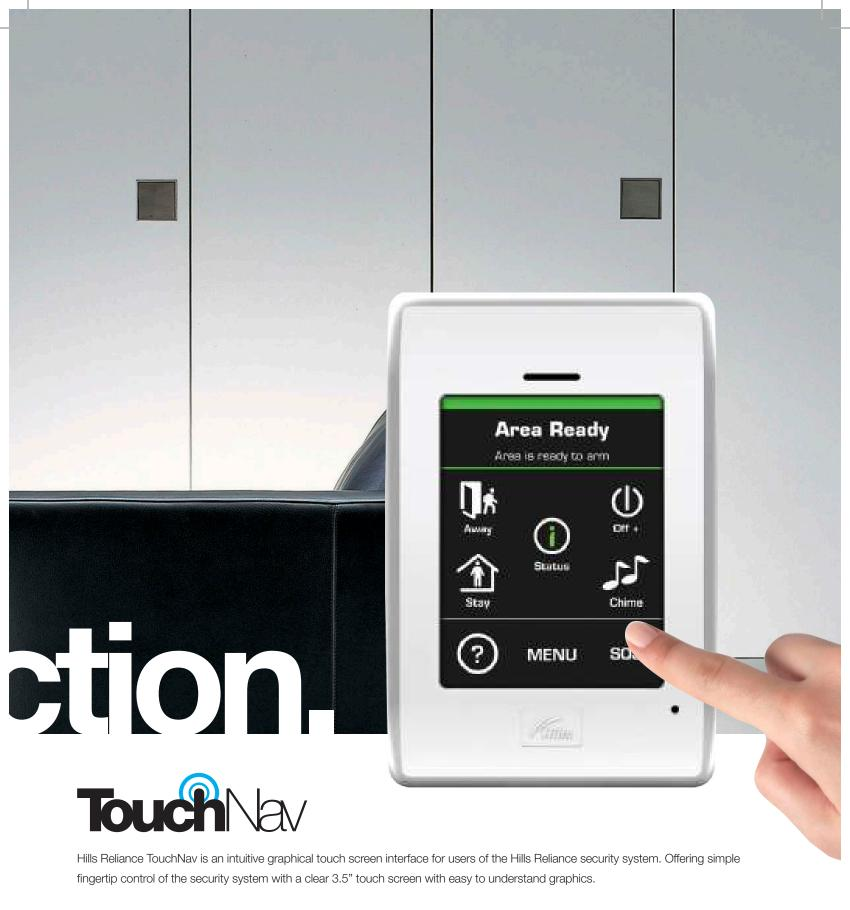
It can be customized for each location when it is installed. This includes custom naming of zones, areas, users and output names. Users can even leave messages for other users via the internal message centre. With the Hills Reliance TouchNav, security is just a touch away.
