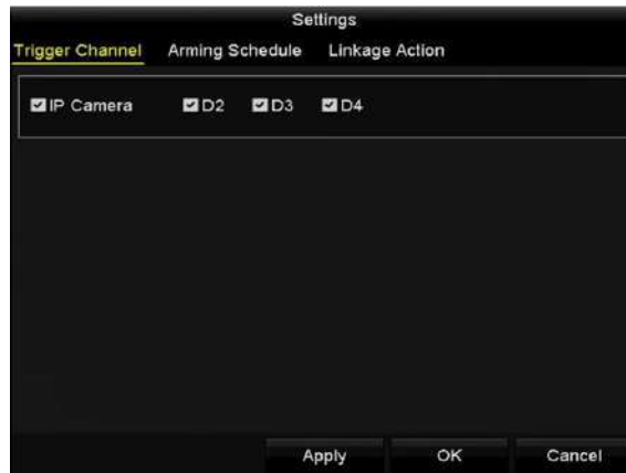
Figure 5-18 Set Trigger Camera of VCA Alarm
