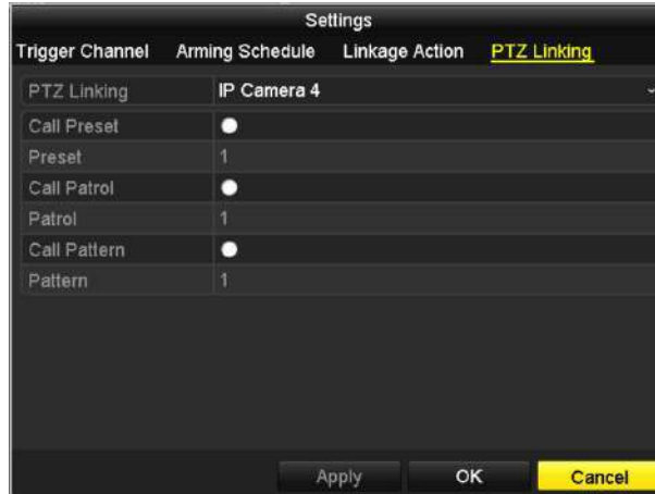
Figure 8-7 Set PTZ Linking of Alarm Input
