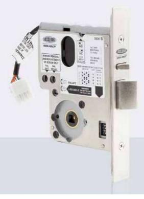
Designed and manufactured in Australia, the 3579HS series electric mortice is designed for unique applications where fail secure functionality is required externally with fail safe functionality on the inside. To achieve this function the lock must be used in conjunction with an electric strike.
