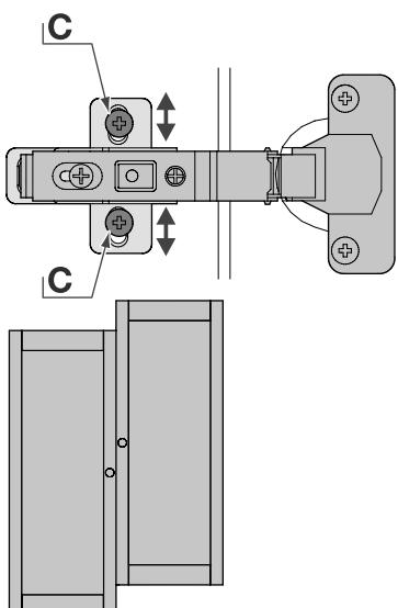
Adjusting the height of the doors. Loosen screws 'C' then slide the hinge plates up or down until the doors are even then tighten the screws.
