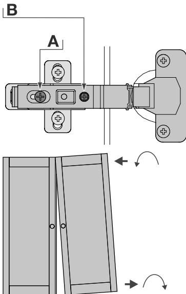
Adjusting the gap between the doors. Loosen screw 'A' slightly. Turn screw 'B' clockwise or anti-clockwise until the gap between the doors is equal, then tighten screw 'A'.
