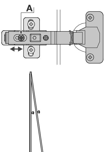
Adjusting the angle of the door. Loosen screw 'A' and slide the hinge arm either forwards or backwards until the door is vertical then tighten screw 'A'.
