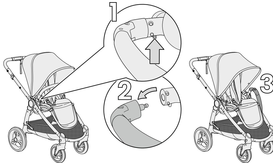
Removing the seat unit – Forward facing
