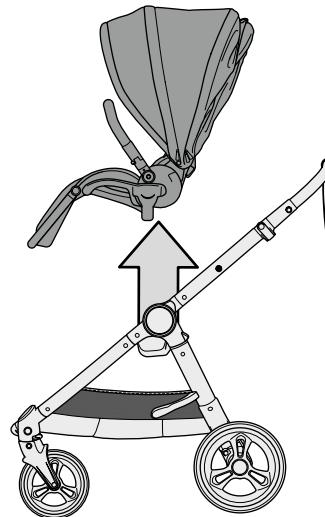
Removing the seat unit – Parent facing
