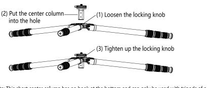
Note: This short center column has no hook at the bottom and can only be used with tripods of a specific model. Mount the center column to the tripod as shown in the image above.
