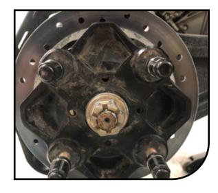
Remove rotor-hub assembly and rotor screws.
