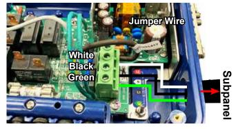
To convert, remove the cord from the terminal block and replace with White, Black and Green #10 wires and connect to 30 amp GFCI Subpanel.
