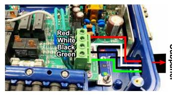
To convert, remove the cord and jumper wire from the terminal block. Remove other end of jumper wire from connector and remove from box. Place Red, White, Black and Green #8 wires onto terminal block and connect other end to 50 amp GFCI Subpanel.
