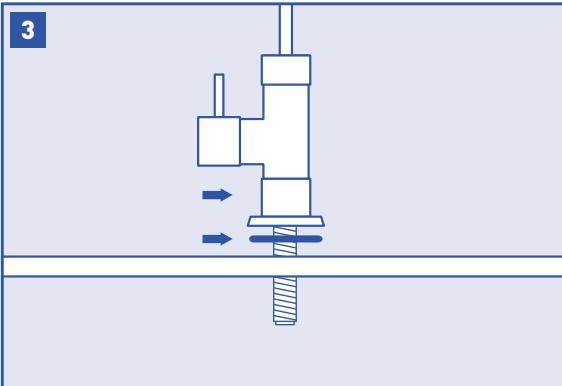
Guide the faucet base gasket onto the faucet base and then onto the faucet. Lower faucet stem through hole in sink. Make sure the faucet sits flat on top of the sink or countertop surface.
