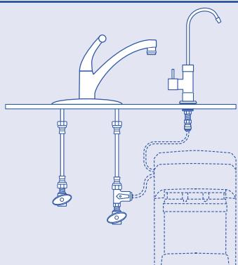
Choose an easy-to-access area under the sink to mount the filter system.
