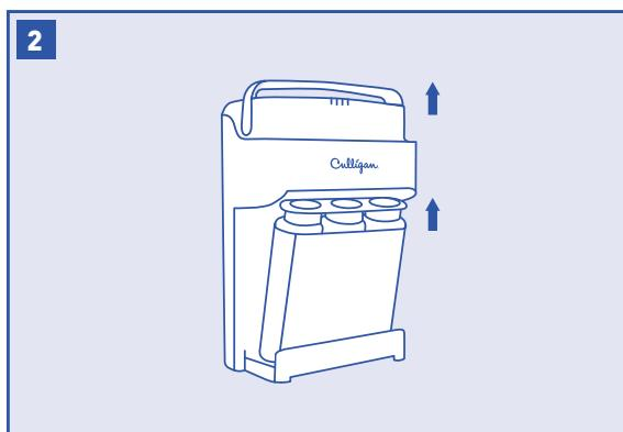
Unlock the system by raising the system handle. Rock the top of the cassette forwards away from the system, then gently remove cartridge from system and discard.
