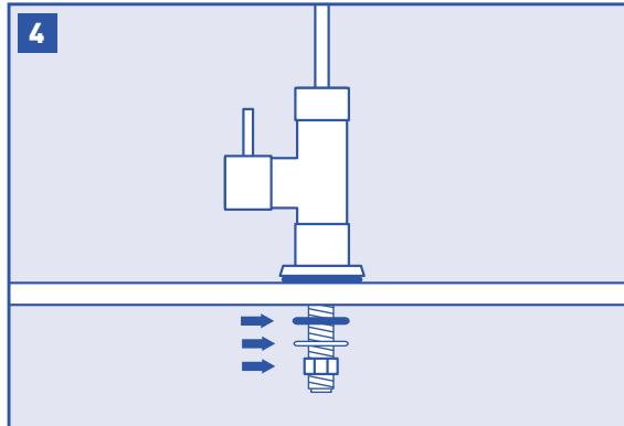
From underneath the sink, guide the black washer onto stem, followed by the metal lock washer, then screw the faucet stem nut all the way up the faucet stem and tighten to secure faucet to sink.
