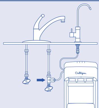
Turn on the cold water shut-off valve and the water supply adapter. Check for leaks.
