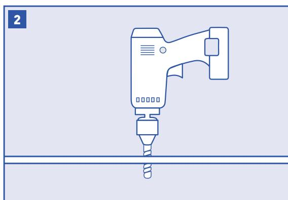
Using a pencil, mark the drill hole. Drill a hole for faucet (most sinks have 1-3/8" or 1-1/2" diameter holes). Drill completely through the sink or countertop.
