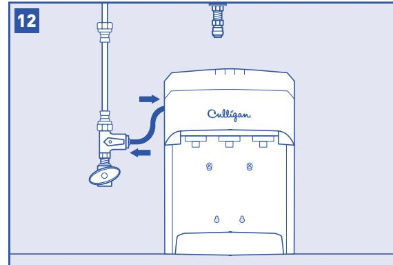
Wet one end of the blue 3/8" plastic tubing with water and push it into the water supply adapter approximately 5/8" until it stops.
