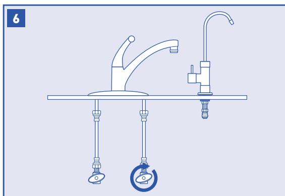
Turn off cold water shut-off valve then turn on the kitchen faucet and allow all water to drain from line.
