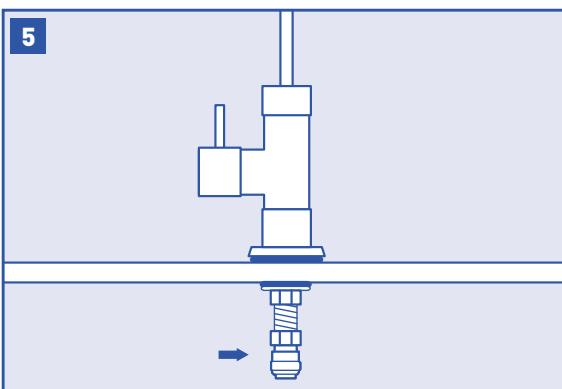
From underneath the sink, hand-tighten the faucet quick connect fitting onto the faucet stem.
