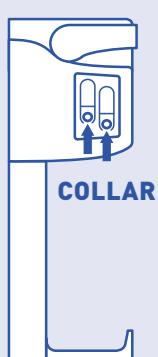
**NOTE:** Routine maintenance and cartridge replacement will not require that you disconnect the tubing from the system head; however, tubing may be quickly and easily removed from the fitting if necessary. First, turn off the water supply to the filter. Open kitchen faucet, then press in the collar around the fitting while pulling the tubing with your other hand.
