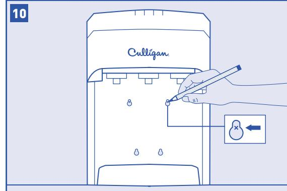
Using the built-in bracket on the back of the system, mark with a pencil the middle of the holes for the mounting screws on the wall surface.
