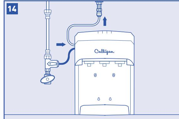
Wet one end of the white 3/8" plastic tubing with water and push it into the faucet quick connect fitting adapter approximately 5/8" until it stops.
