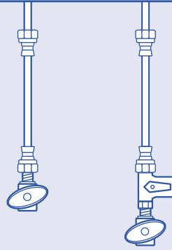
Hand-tighten the water supply adapter to the cold water shut-off valve as shown.
