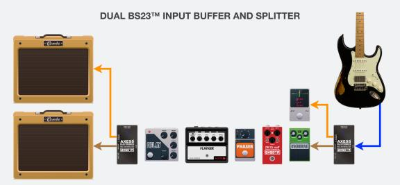
Some (older/old-school) tuners are noisy and a rig can benefit not only from having the tuner out of the signal path, but also from feeding it with an audio isolation transformer. This prevents the tuner's noisy ground currents from getting into the audio signal path.
