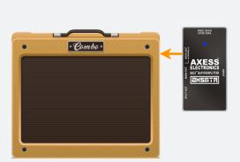
A ground loop occurs when an amp(s)/rig sees more than one path to (earth) ground, as is the case when running multiple amplifiers and/or other devices/effects that are grounded via a 3-prong AC-plug, and results in an audible and annoying 60 cycle hum.
