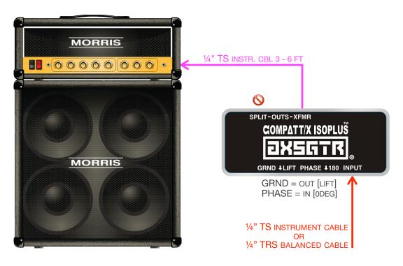
The ideal location for the IsoPlus<sup>TM</sup> is close to the backline amplifier and its input requires a buffered instrument level guitar signal, i.e. a pedalboard with either an always on last pedal, a Compatt/O<sup>TM</sup> Buffer, or a Compatt/X<sup>TM</sup> Unity+<sup>TM</sup>. When using standard  $\frac{1}{4}$ " TS (tip-sleeve) instrument cables — always aim for the best quality and shortest length possible.
