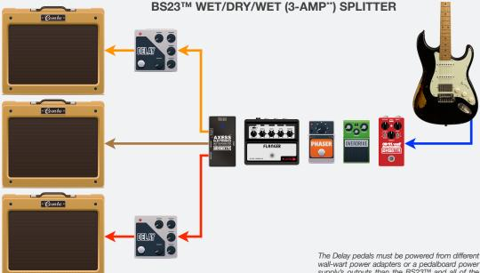
" Fitting the SPLIT OUT with an optional isolation transformer allows the BS23™ to feed 3 amps.
