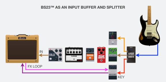
Some (older/old-school) tuners are noisy and a rig can benefit not only from having the tuner out of the signal path, but also from feeding it with an audio isolation transformer. This prevents the tuner's noisy ground currents from getting into the audio signal path.
