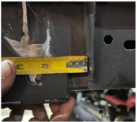
IMPORTANT: Please double check this distance for your winch. Different winches may require different spacing of the install. This measurement works for most BUT NOT ALL of Warns winches\*
