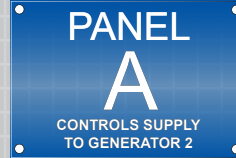
Nameplate Size: 2 x 3 in Row one - 3/8 in text size Row two - 3/4 in text size Row three and four - 3/16 in text size
