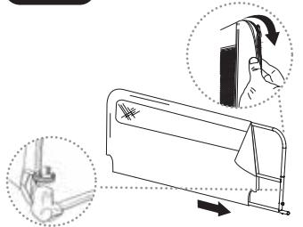
To install the mesh wall (A) on the bed rail, slide it over the frame until it reaches the other end, zip it shut, then attach the velcro strap over the zipper to complete the installation. Repeat STEPS 1 – 3 to assemble the second side of the double bed rail. Mesh wall must go over entire bed rail frame.
