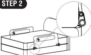
Once the bed rail is placed properly, place the mattress back atop of the box spring or mattress support, sandwiching the flat metal bars on the corner hinges and the anchoring straps between the box spring and the mattress.
