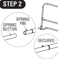
With the upper and bottom support bars assembled, connect the two sides.
