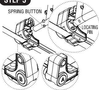
Insert one side of the wall frame with locating pin into the hinge assembly labeled "B". Press in the metal spring button to fully insert the tube into the hole in the plastic hinge. The spring button should line up with the access hole in the plastic sleeve on the hinge. The spring button will rebound and lock the tube in place. Repeat on opposite hinge assembly "A". Repeat steps 1-5 to assemble opposite bed rail side.
