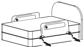
Tighten the straps to bring the bed rail into its proper position. To tighten the straps, first release the strap locks on the under side of the plastic hinges. Pull the straps towards you until all the excess slack has been pulled out from under the mattress and both sides of the bed rail are firmly pressed against the sides of the mattress.
