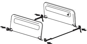
With the wall of the bed rail completely assembled, you will now connect the hinge assemblies (F, G).
