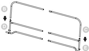
Insert the upper support bar (C) into the bottom support bar (E). Make sure the spring pin fits securely into the opposing hole so that the two pieces cannot pull apart. Repeat on the opposite side (B, D) of the bed rail.
