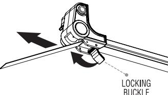
If the strap does not pull through smoothly, the strap may be twisted under the mattress. Correct this before continuing with the installation. Once you have taken the slack out of the straps, give one final pull on the strap end, hold it, and push down on the locking buckle to secure the strap tension. Use the same procedure for each side to properly secure the bed rail.
