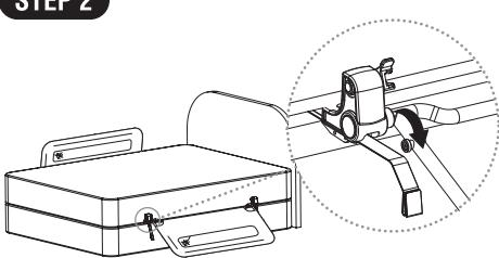
With both locking tabs turned to the 'open' position, hold the upper part of the bed rail firmly and swing it down. The bed rail should now be in the 'down' position. To return the bed rail to the 'up' position, reverse STEPS 1 – 2.
