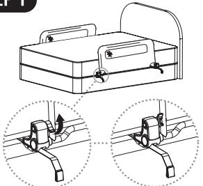
With the bed rail side in the 'up' position, release the locking tabs on each swing lock and arm assembly by pushing them up. This will allow the upper part of the bed rail to move freely.
