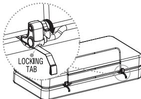
With your bed rail in the 'up' position push down on the locking tabs to secure your bed rail in place.
