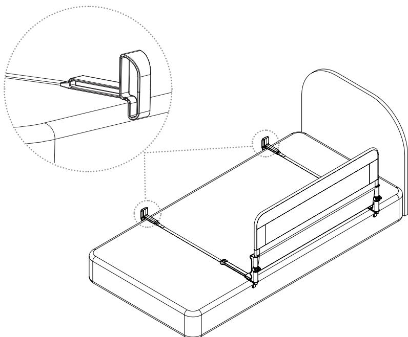
**NOTE:** You may need to release the strap locking buckles located on the under side of the plastic hinges. Ensure that the large end of the anchor is pointing up. The anchoring straps should not be twisted. If twisted, the anchoring straps will not tighten properly.
