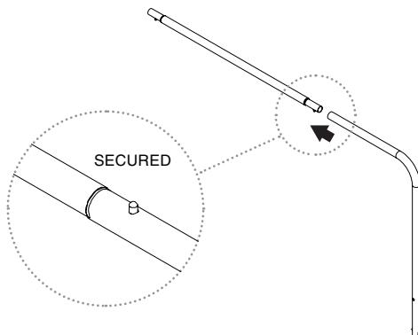
**NOTE:** Make sure that the spring pins are secured into the opposing holes so that the bed rail cannot pull apart.
