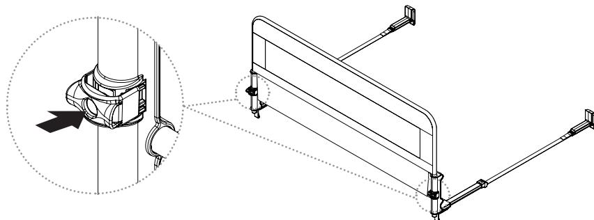
**NOTE:** The top of both plastic flanges must rest against the bottom of the mounting bracket.
