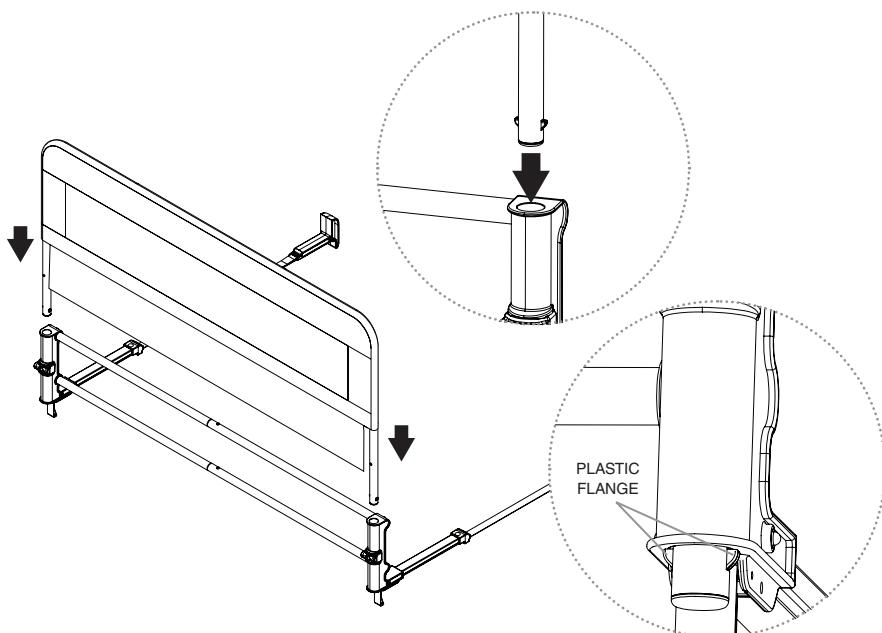
**NOTE:** Lower rail assembly locks must be in the “unlock position” to insert upper and lower rail assembly.
