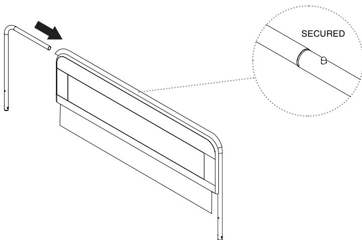
**NOTE:** Make sure that the spring pins are secured into the opposing holes so that the bed rail cannot pull apart.
