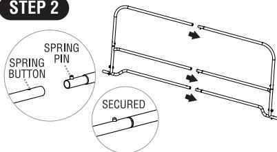
With the upper and bottom support bars assembled, connect the two sides.
