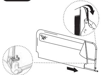
To install the mesh wall (A) on the bed rail, slide it over the frame until it reaches the other end, zip it shut, then attach the velcro strap over the zipper to complete the installation. Mesh wall must go over entire bed rail frame.
