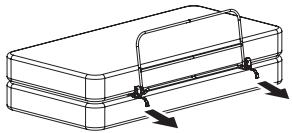
Tighten the straps to bring the bed rail into its proper position. To tighten the straps, first release the strap locks on the under side of the left and right under bars. Pull the straps towards you until all the excess slack has been pulled out from under the mattress.
