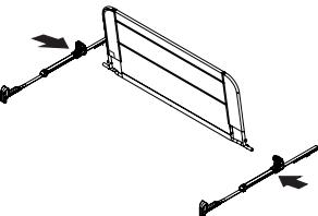
With the wall of the bed rail completely assembled, you will now connect the hinge assemblies (F, G).
