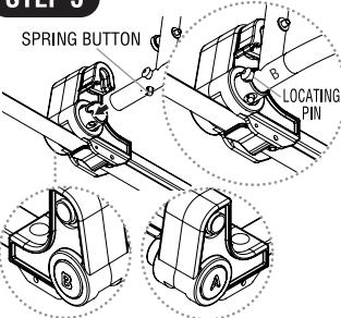
Insert one side of the wall frame with locating pin into the hinge assembly labeled "B". Press in the metal spring button to fully insert the tube into the hole in the plastic hinge. The spring button should line up with the access hole in the plastic sleeve on the hinge. The spring button will rebound and lock the tube in place. Repeat on opposite hinge assembly "A".
