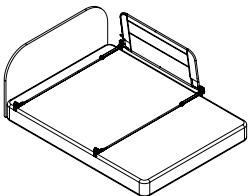
Start by placing the bed rail on the side of the bed you have chosen for installation. The left and right swing lock and strap assemblies should be placed on top of the box spring that will support the mattress. The 'T' shaped anchors and straps should be extended opposite the bed rail and mounted to the outer edge of the box spring or mattress support structure.
