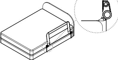
Once the bed rail is properly placed, check to make sure the left and right swing lock and strap assemblies are parallel to one another. Then, place the mattress on top of the assembly.
