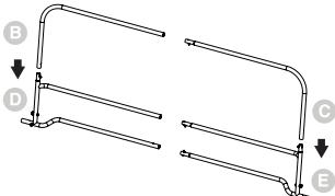
Insert the upper support bar (C) into the bottom support bar (E). Make sure the spring pins fit securely into the opposing hole so that the two pieces cannot pull apart. Repeat on the opposite side (B, D) of the bed rail.
