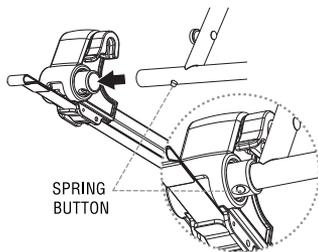
Insert one side of the wall frame into one of the leg pieces. Press in the metal spring button to fully insert the tube into the hole in the plastic hinge. The spring button should line up with the access hole in the plastic sleeve on the hinge. The spring button will rebound and lock the tube in place. Repeat to complete the assembly of the other leg.
