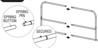
With the upper and bottom support bars assembled, connect the two sides.
