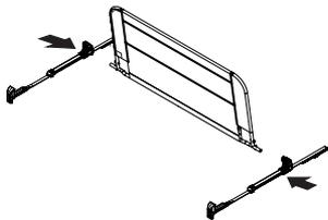
With the wall of the crib rail completely assembled, you will now connect the left (G) and right (F) hinge assemblies.
