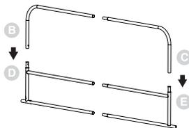
Insert the upper support bar (C) into the bottom support bar (E). Make sure the spring pin fits securely into the opposing hole so that the two pieces cannot pull apart. Repeat on the opposite side (B, D) of the crib rail.
