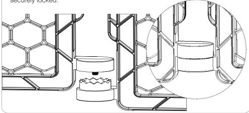
Attach two *gate connectors* to one of the free ends of your gate at the specified *mounting locations* shown below. The placement of the *gate connectors* will determine where your gate is attached to the wall. Repeat step for the other free end of the gate.
