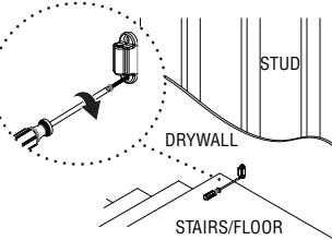
Using the supplied 2" wood screws (I), screw through the lower mount wall hinge into the drywall and stud. Do this for the top and bottom hole.
