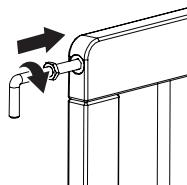
Screw the top hinge adjuster knob (G) into the main gate panel (A). Repeat with the lower knob as well. Rotating the hinge in the clockwise direction will bring the hinge in. Loosen the jam nut all the way back.
