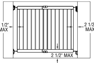
When the gate is in the closed and latched position there should be no larger than a 2 1/2" gap from the wall to the first picket on either side. To achieve this either screw inward or outward the hinge adjustment knobs and/or the receiver adjuster knobs.
