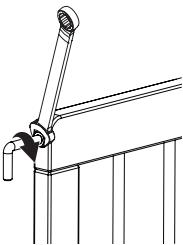
Once the 2 1/2" maximum gap is set, tighten down the 4 jam nuts with a 13mm wrench. One on each hinge adjustment knob and one on each receiver adjuster knob.
