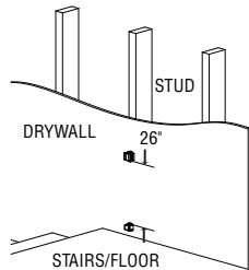
Repeat with the wall mount hinge snap female (B). The distance between the top hole of the lower mount wall hinge and the lower hole of the wall mount hinge snap female is 26".
