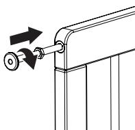
Screw the top receiver adjustment knob (H) into the second gate panel. Repeat with the lower knob as well. Rotating the receiver in the clockwise direction will bring the receiver in. Loosen the jam nut all the way back.
