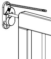
With the gate in closed position (creating a 90° angle to the wall the hinges are on) place the receiver adjustment knob in the latch assembly wall mount (D). Mark the location of the holes, making sure you are located on top of a stud. Do this for the upper and lower receiver.
