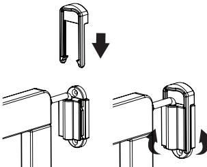
Install the wall mount hinge snap female over the wall mount hinge snap male. Do so by matching the "legs" of the wall mount hinge snap female over the grooves, and sliding down until it clicks into place of the wall mount hinge snap male (C).
