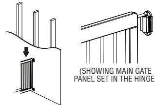
Place the main gate panel with the hinge adjuster knobs into the upper and lower hinges on the wall. Press the main gate panel in a downward motion to set the hinge adjuster knobs into the hinges.
