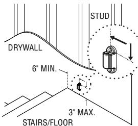
The hinges get installed on the right side of the stairs (when looking down the stairs). Using a stud finder locate a stud in the wall that is at a **minimum** 6" from the edge of the top stair. Once the stud is located, place the lower mount wall hinge (E) against the wall. Position it so the upper hole of the lower mount wall hinge is at a **maximum** of 3" above your floor.
