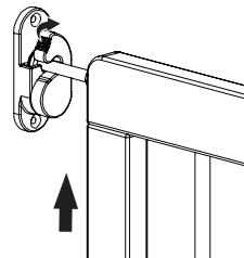
To open the gate. Rotate the latch of the latch assembly wall mount in the clockwise direction to release the gate. Lift the gate upward and away from the stairs. Pivot the gate in the hinges until fully open.
