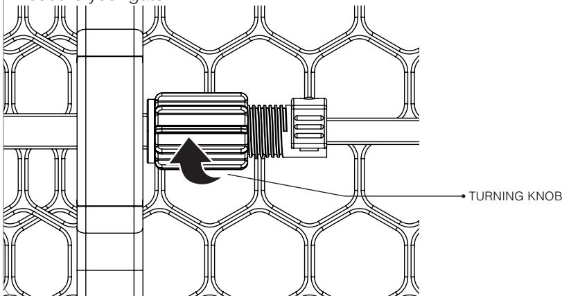
**NOTE:** Test the gate to make sure it is tightly secured and cannot be easily pushed out.
