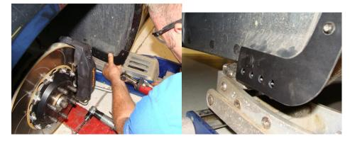
The outside mounting hole in the stone guard is over-size, therefore, allowing you to position the stone guard according to taste. As an example, you can change the horizontal position to alter the amount of the stone guard seen from the side or the car.
