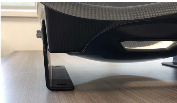
Showing the two degree camber and set on the upper holes without spacers
