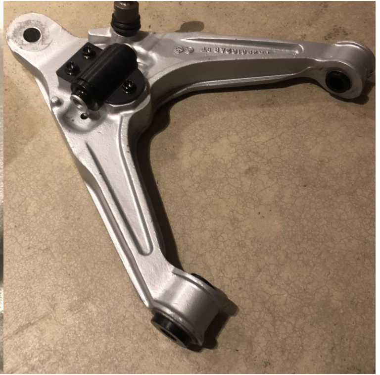
Lower Shock Mount Bushing Installed In Lower Control Arm
