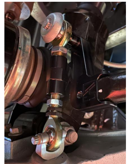
Installed Link with Preferred Orientation
