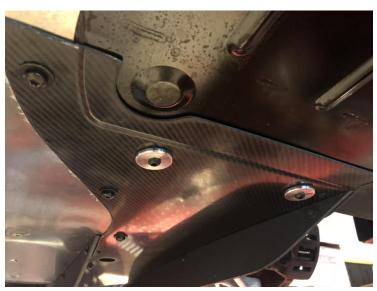
Diffuser Hard Mount Installed (Shown Not Anodized)
