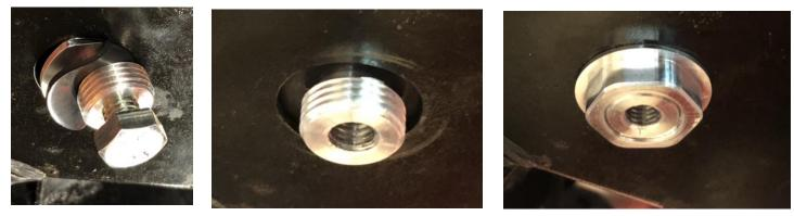
Diffuser Hard Mount Upper Boss Assembly Installation Progression (left to right)
