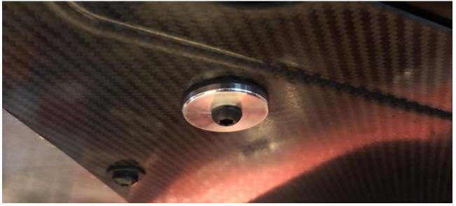
Hard Mount Completely Installed Showing Gasket Centered On The Washer.
