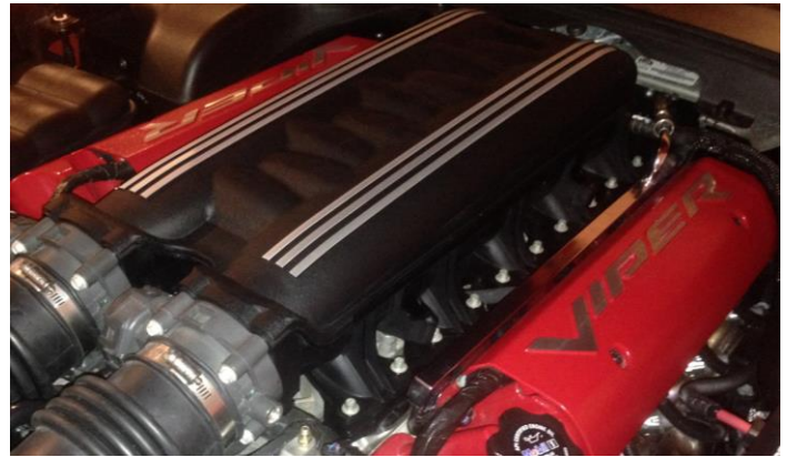
Gen V manifold installed using DSE Compression Limiters
