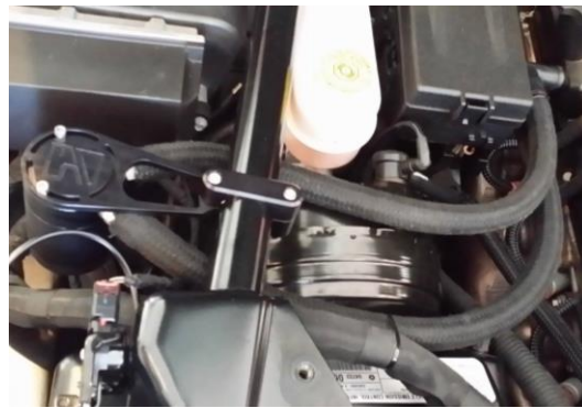
Dual Sealed Catch Can Setup Installed on Passenger Side (Left) and Driver Side (Right)
