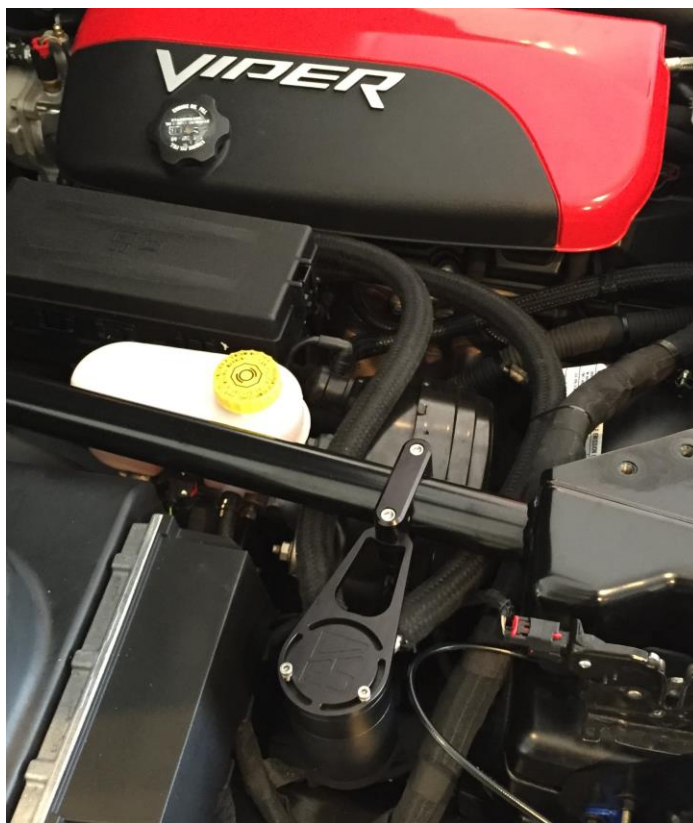
Catch can install (sealed driver side)
