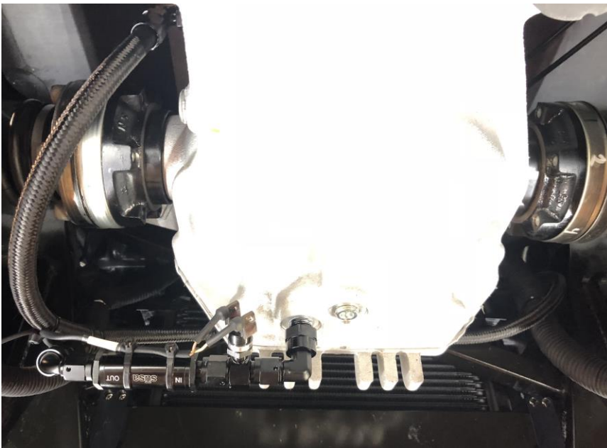
Differential Cooler Exit Wrapping Around Wiring Harness and Tied to the Filter Leg To Secure the Hose Away from the Halfshaft
