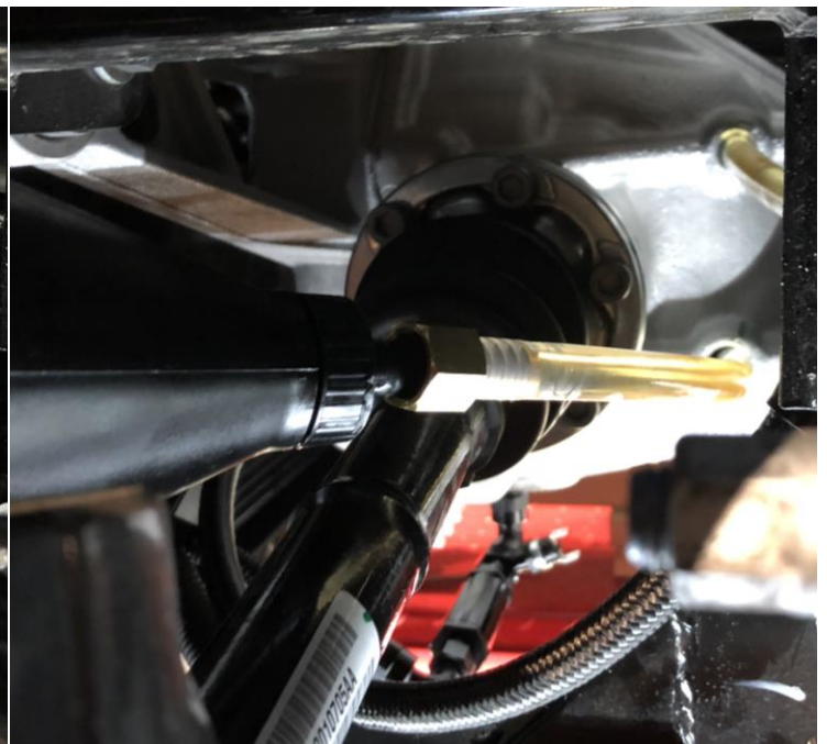
Wheel Well View of Priming the Differential Pump (left) and Filling the Differential via the Fill Port (right) Using the Upper Cooler Exit Hose
