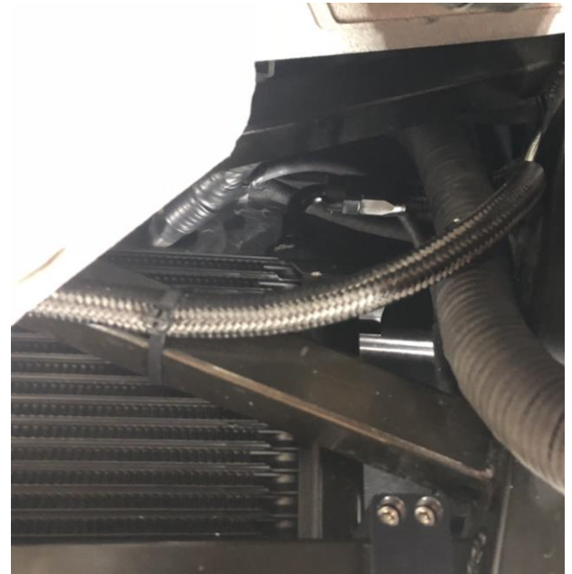
Differential Cooler Exit Wrapping Around Wiring Harness and Tied to the Filter Leg To Secure the Hose Away from the Halfshaft
