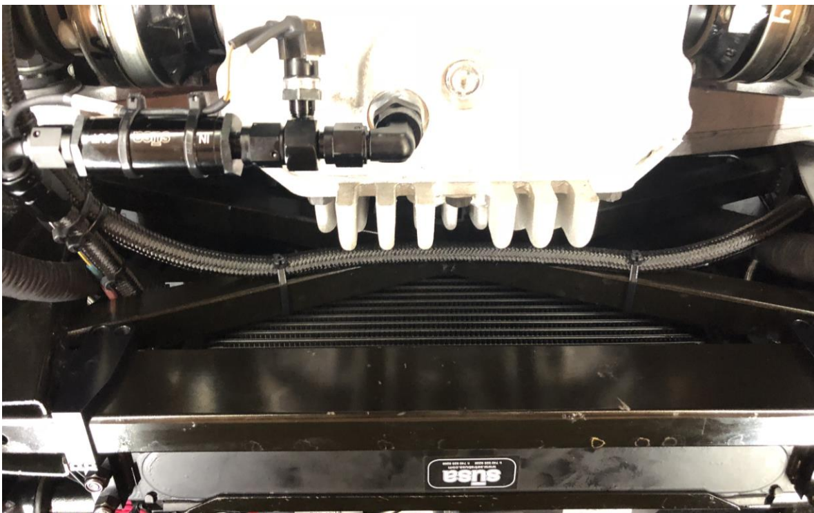
Differential Cooler Exit Hose Crossing The Frame
