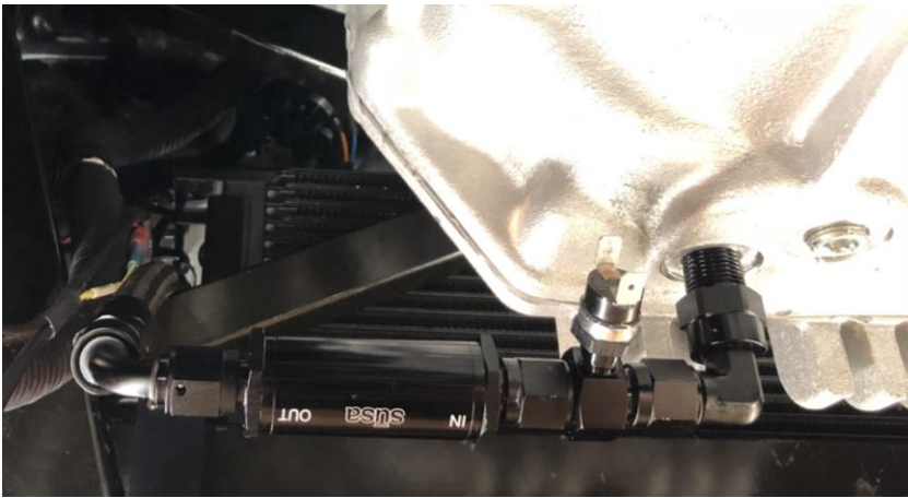
Differential Filter / Switch Leg Installed (left) and Differential Pump Exit / 190 / 200 Switch Leg Orientation (right)
