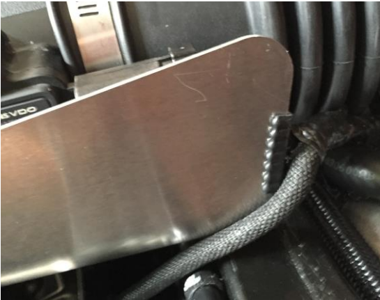
Anti-abrasion edging installed (Gen IV Only)
